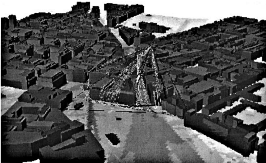
Figure 11.6 An example of ray tracing. It shows the dominant rays for the pixels along a line just in front of a row of buildings. Notice the vertical, transversal and reflected components (Courtesy Mobile Systems International plc).
