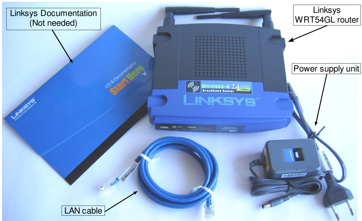
Figure 7: Linksys WRT54GL and package contents
