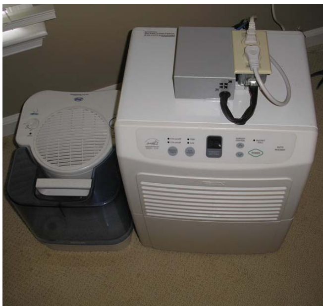
Figure 6. Completed Humidity Controller with Humidifier and Dehumidifier Connected
