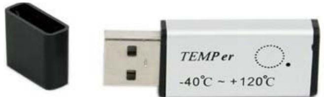
Figure 1. TEMPer USB Thermometer (photo from the Amazon product page)
