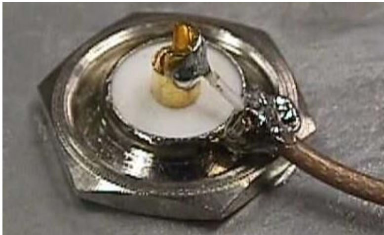
Filter's RF output N-connector. Yes, this is incorrect construction at those high microwave frequencies, but I didn't have a choice.
