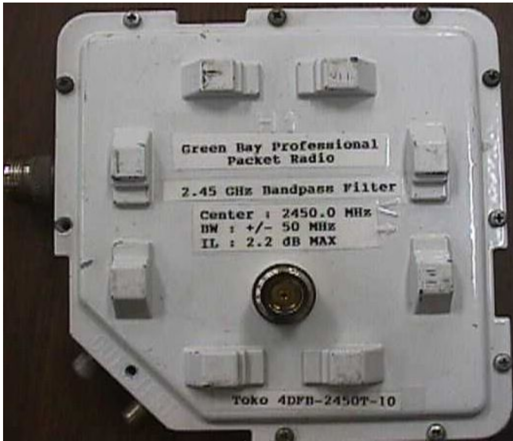
Overview of an (optional) external 2.45 GHz band pass filter which can be placed ahead of the downconverter to reduce out-of-band interference and intermodulation products. The case is from another California Amplifier downconverter.
