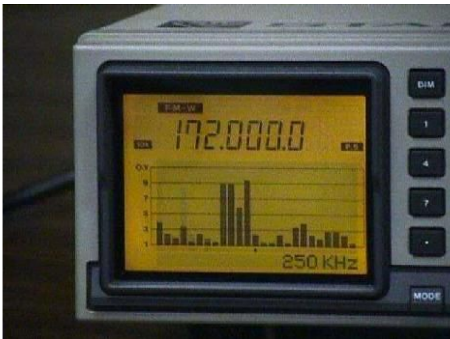
Microwave oven leakage is observed! The 2.45 GHz oven RF radiation is mixed with the downconverter's internal 2.278 GHz LO signal and then converted to 172 MHz. Microwave ovens tend to drift slightly in frequency, as the spectrum display shows.
