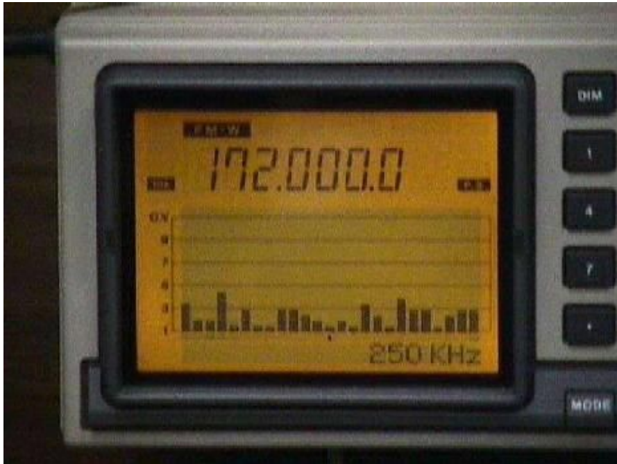
Noise floor shown at 172 MHz while connected to the powered MMDS downconverter.
