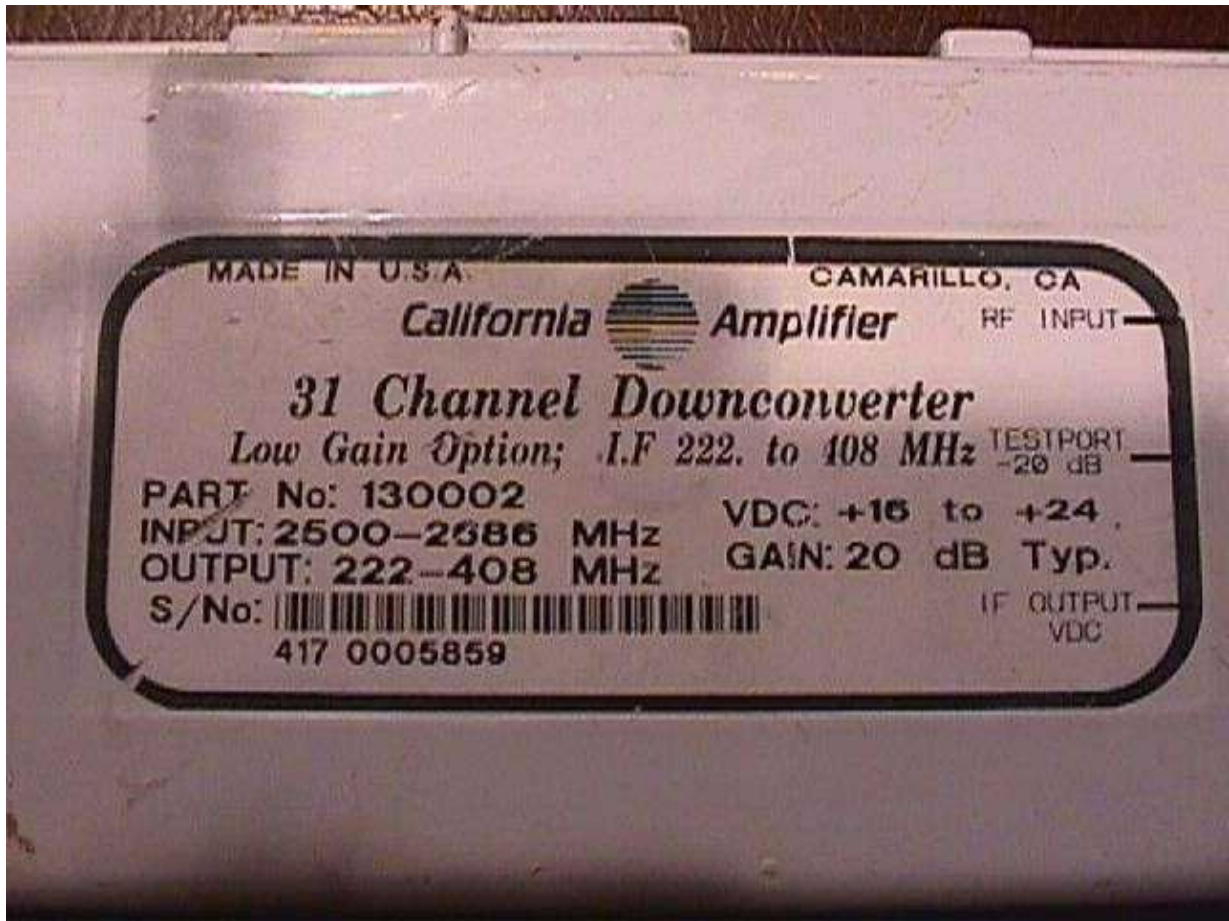
Case label on a dumpster-dived CalAmp MMDS downconverter.
